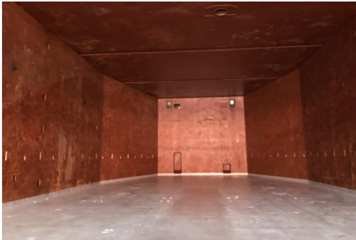
Hold looking forward Showing narrowing over 8.1 m to 8 m
