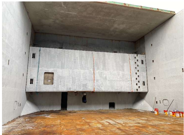
Hold looking forward Showing bulkhead stowing position
